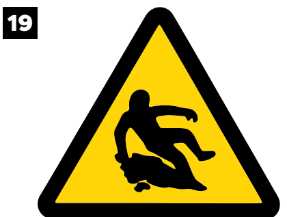
19 Slip hazard label/decals. Fitted adjacent to the tailgate/doors at the rear of the trailer, and on the ladder and platform. May also be fitted in other positions.
