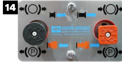
14 Fitted to the left side of the chassis adjacent to the parking brake control.
